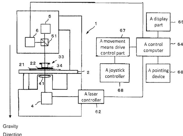
the dissection laser light and positional coordinates of the thermofusible film in a location where the collected sample is adhered, and a movement means drive control part for controlling driving of the sample movement means and the device movement means on the basis of the positional coordinates of the sample and the thermofusible film. The dissection laser light is radiated through the device onto the sample from below the device.
