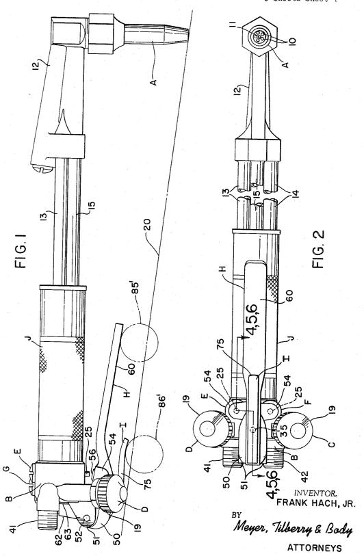
VALVE CONTROL MECHANISM FOR GAS TORCHES
