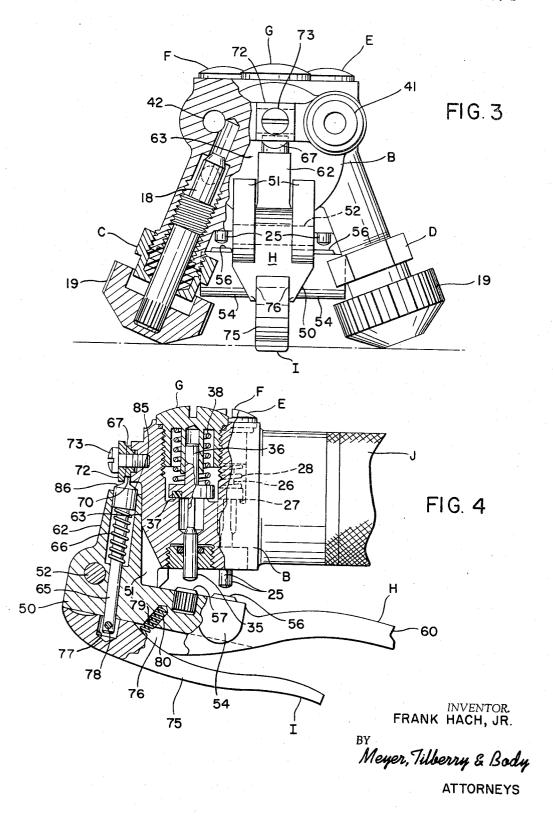
VALVE CONTROL MECHANISM FOR GAS TORCHES
