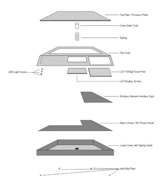
Figure 2: Firearm Alarm Parts Breakout
