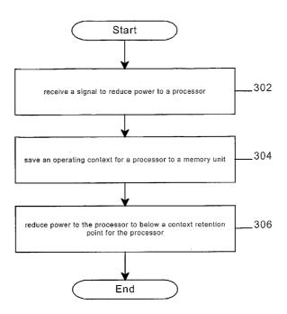
(57) Abstract: System, apparatus, method and article to manage power for a mobile device are described. The apparatus may include a power management module to save an operating context for a processor to at least one memory unit, and reduce power to the processor below a context retention point. Other embodiments are described and claimed.
