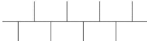
Polypropylene having this type of chain configuration is called syndiotactic polypropylene, or sPP.
