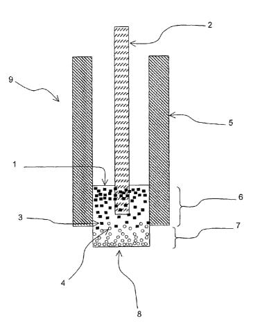
(57) Abstract: Potentiometric electrode and gradient polymer, both comprising electrically conducting particles, which increase in concentration away from one surface, ionophore molecules, which increase in concentration towards the same surface surface, and an electrical connection which passes proximal to said electrically conducting particles. Devices incorporating said electrode or gradient polymer, and to a method for their preparation. The new materials are highly robust and reliable.
