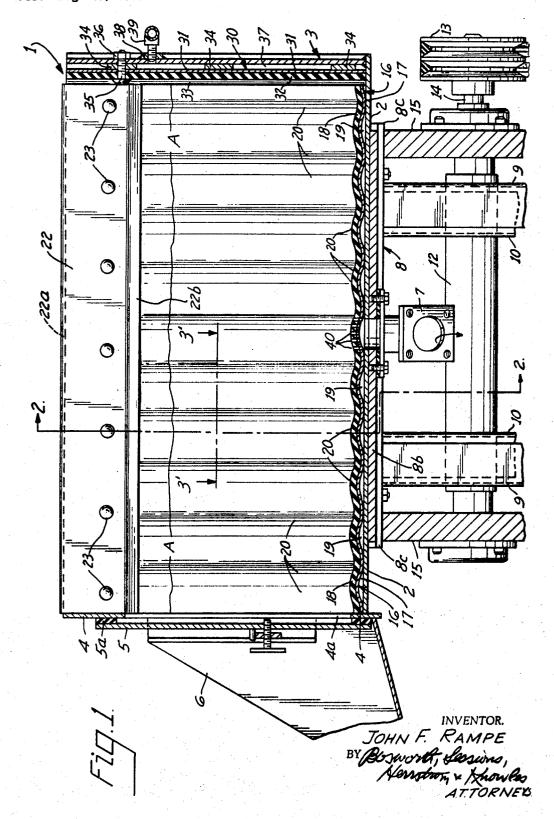
LIQUID-COOLED PROCESSING VESSEL
