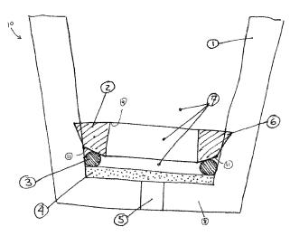
face, the surface of the compression element, and the well wall in a liquid-tight manner. The compression element may be configured so that it is fixed in the well such as by an interference fit with the well wall or by bonding to a surface of the substrate.
