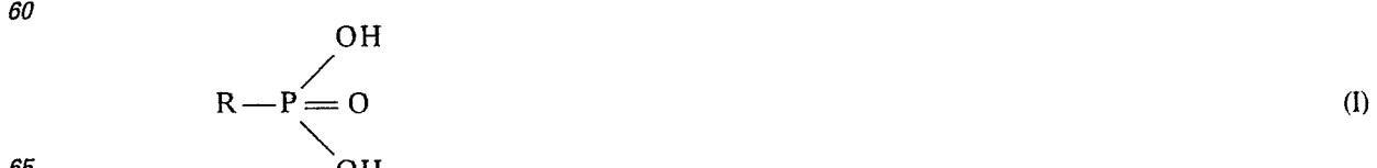
in which R means a linear alkyl radical having from 6 to 24 carbon atoms, or with an alkane phosphonic acid monoalkyl ester of the formula (II), in an amount of from 0.1 to 5 percent by weight (relative to the amount by weight of the vinyl monomers) and, optionally, up to 10 percent by weight (relative to the dispersion) of usual additives are added to the dispersion.
