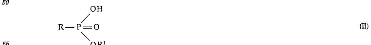
55 in which R means a linear alkyl radical having from 6 to 24 carbon atoms and R<sup>1</sup> represents an alkyl radical having from 1 to 8 carbon atoms, or a mixture of such a salt with an alkane phosphonic acid of the formula (I)
