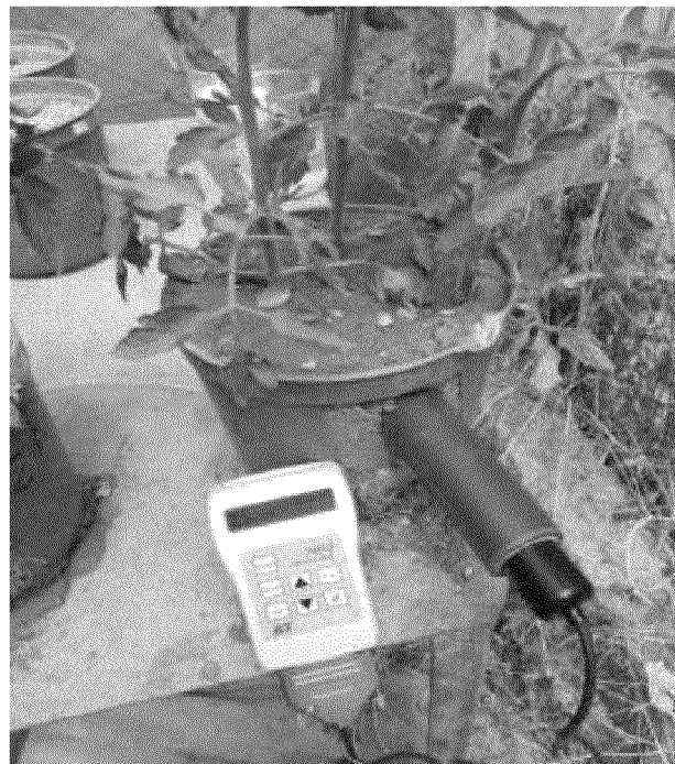
Figure 5 : Soil moisture measurement above beads layer.
