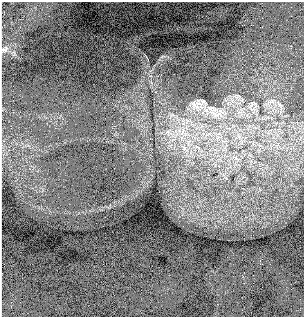
Figure 12: Effect of beads on water evaporation
