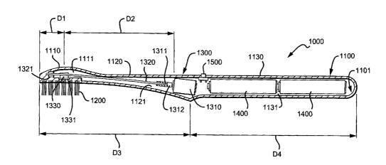
(57) Abstract: A vibratory toothbrush having a handle (1130) supporting a head (1110) via a neck (1120). A rotating eccentric weight (1330) positioned in or near the head (1110) of the toothbrush to cause movement of the head.
