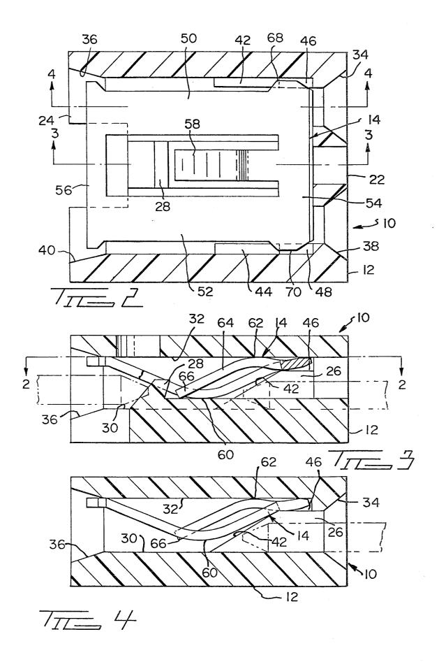
The present invention relates to a shunt connector and in particular to a shunt connector which cannot be 5 improperly mounted on a pair of adjacent pin terminals.
