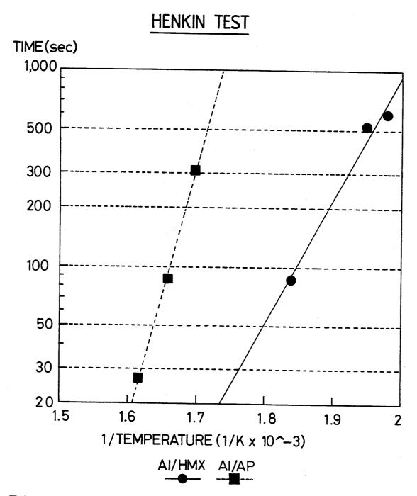
Filled points indicate reaction ca 100mg SAMPLES
