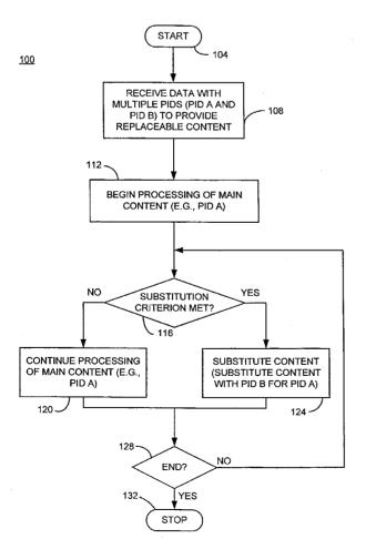
(57) Abstract: A method and encoder for substituting content which comprises receiving data with multiple PIDs to provide replaceable content (108), processing of main content (112), determining if a substitution criterial has been met (116), and substituting main content with secondary content (124).
