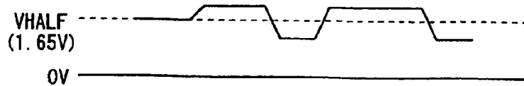
FIG. 5 (c) EXAMPLE OF WAVEFORM OF VOLTAGE ACROSS SPDRV AND VHALF (VOLTAGE DIVIDING RESISTOR IS ON)
