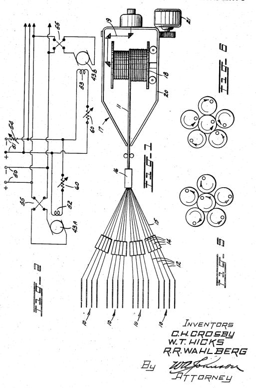
APPARATUS FOR MAKING RANDOM UNIT LAY CABLE
