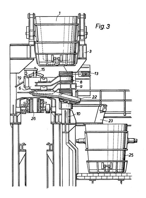
APPARATUS FOR MOLTEN METAL SUPPLY CHANGEOVER DURING CASTING
