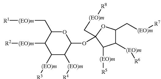
[0152] R<sup>1</sup>, R<sup>2</sup>, R<sup>3</sup>, R<sup>4</sup>, R<sup>5</sup>, R<sup>6</sup>, R<sup>7</sup>, and R<sup>8</sup> can be any combination of H, hydrocarbon, polyoxyalkylene, siloxane or fluorinated groups. The method of functionalizing the polyol may be, but not limited to esterification, etherification, amidation and other linking chemistries.
