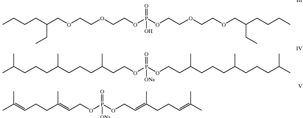
**[0116]** In some embodiments, the composition comprises from about 0.01 to about 10 wt % of a phosphate based surfactant, from about 0 to about 20 wt % of water, from about 0.1 to about 20 wt % of other detergent adjuncts, and the balance of lipophilic fluids. These cleaning compositions have been shown to enhance the overall cleaning and stain removal performance of the composition. These compositions are particularly effective in the cleaning and removing stains of blood, grass and tea.
