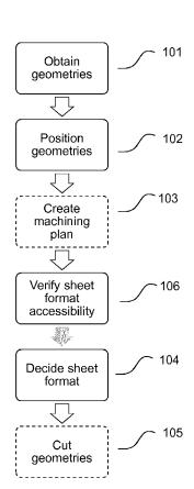
(57) Abstract: The invention relates to a method (100) for preparing machine cutting in sheet material, comprising the steps of obtaining (101) a set of geometries to be cut, positioning (102) the set of geometries for cutting, and thereafter deciding (104) on a format of sheet material based on the positioned geometries. The invention further relates to a corresponding system for machine cutting in sheet material, and a corresponding computer program product.
