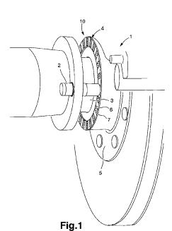
(57) **Abstract**: The invention relates to a vehicle speed sensor arrangement 1 comprising a stationary sensor 2 placed in front of a rotatable sensor wheel 4. The sensor wheel 4 is concentrically mounted on a rotatable wheel hub 5 wherein the rotatable sensor wheel 4 having a surface facing the stationary sensor 2, the surface having circumferentially arranged alternating magnetic segments 6, 36 and non-magnetic segments 7, 37.
