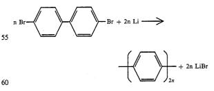
The ultrasonic-promoted coupling reaction is conducted under an inert atmosphere, such as moisture-free nitrogen, helium, or argon.
