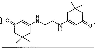
A mixture of 6.04 g ethylenediamine and 31.15 g dimedone in 200 ml toluene is heated under reflux conditions using a water separator for three hours.
