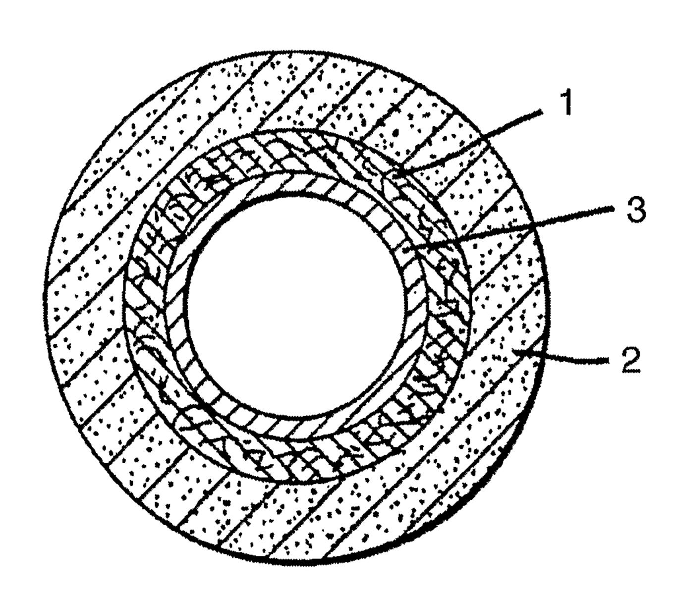
(57) Abstract: An orthopedic cast system, including a hydrophilic inner layer; a hydrophobic outer layer having opposing surfaces adjacent to said hydrophilic inner layer, wherein the hydrophobic layer has an apparent surface energy less than about 60 dynes per centimeter; and a curable casting material disposed on one of the opposing surfaces is provided. Additionally, a method of immobilizing a body part is provided. An orthopedic cast kit is also provided.
