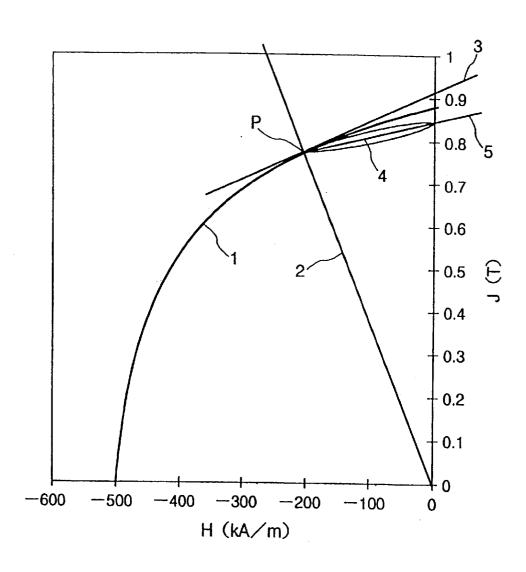
No.1: Demagnetization Curve
