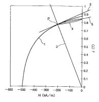
No.1: Demagnetization Curve
