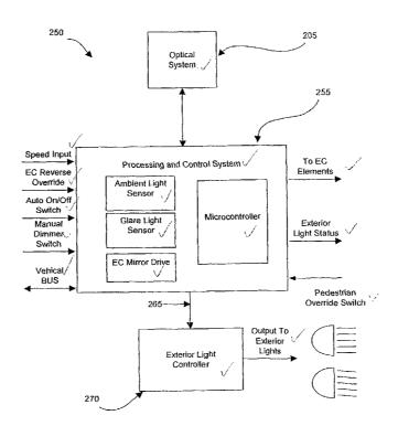
(57) Abstract: The present invention relates to a vehicle light control system (250) configured to distinguish between reflections off of a highly reflective surface and reflections off of atmospheric conditions of interest.
