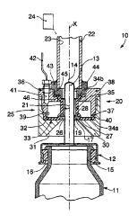
selectively define a reduction in section of the housing channel suitable to hold the spout.
