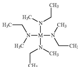
In the chemical formula (2), (3), or (4), M represents a transition metal. Specifically, the transition metal M is Ti, Hf, or Zr. M may also be Sn as other metal which is not the transition metal.
