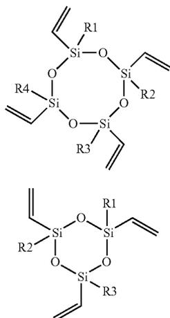
(in which, in the chemical formula (5) or (6), R1, R2, R3, and R4 each represents one of hydrogen, an unsaturated hydrocarbon group, and saturated hydrocarbon group, and each of the unsaturated hydrocarbon group and the saturated hydrocarbon group is a vinyl group, allyl group, methyl group, ethyl group, propyl group, isopropyl group, or butyl group).
