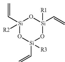
In the chemical formula (5) or (6), each of R1, R2, R3, and R4 is hydrogen, an unsaturated hydrocarbon group, or a saturated hydrocarbon group. Each of the unsaturated hydrocarbon group and the saturated hydrocarbon group is a vinyl group, allyl group, methyl group, ethyl group, propyl group, isopropyl group, or butyl group.
