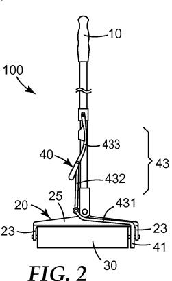
(57) Abstract: A cleaning member mounting holder for a mop is disclosed. The cleaning member mounting holder comprises: a shaft for mounting a cleaning member, the shaft having opposite ends, and a pair of mounting members each having a hole, the opposite ends of the shaft being mounted in the holes of the pair of mounting members respectively, wherein the ends of the shaft are movable substantially perpendicularly to the shaft axis in the holes of the pair of mounting members.
