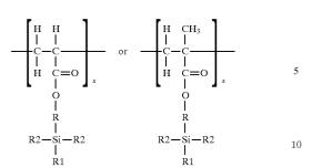
where R1 in each formula is the polydiorganosiloxane moiety —(OSiR2<sub>2</sub>)<sub>z</sub>OSiR2<sub>3</sub>; R2 in each formula is the hydrogen atom, a  $\rm C_{1-8}$  alkyl radical, a haloalkyl radical, or an aryl radical; R in each formula is a divalent hydrocarbon radical with 1–6 carbon atoms; x in each formula is 2–5000; and z in each formula is 1–1,000.
