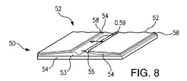
(57) Abstract: A corner bead for wallboard applications comprising a polymeric core having a bonding surface for bonding to wallboard wherein the bonding surface has applied thereto a water activated adhesive which is bonded to the polymeric core by a curable adhesive having embedded therein fibers which are also embedded in the water activated adhesive.
