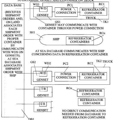
(57) Abstract: A database dispatches data to a wireless device on the particular source that powers a container during any segment of its journey.
