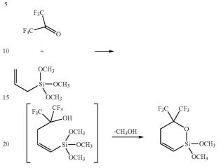
The intermediate in brackets was initially expected to be the product, but the tertiary hydroxyl group derived from the hexafluoroacetone is well-situated to nucleophilically displace one of the methoxy groups on the silicon to eliminate methanol and close the six membered ring. The synthesis, purification and characterization of this compound are
