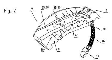
(57) **Abstract**: Climate conditioning device (10) for a climate conditioned object (2), the climate conditioning device (10) having at least one of the following components: a) a temperature control device (70) to heat or cool the climate conditioned object (2), b) an air moving device (57) to generate an air stream to exchange thermal energy with the surrounding.
