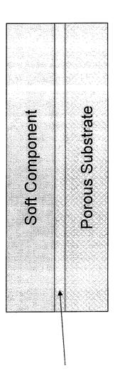
Soft component partially penetrates into porous substrate
