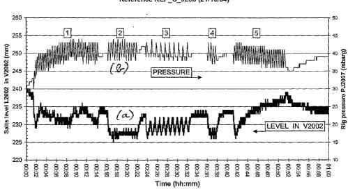
RFD operation with molten salts: variable cycle length Reference REP\_C\_028b (21/10/04)
