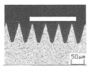
Depth of groove is  $76.7\,\mu$  m
