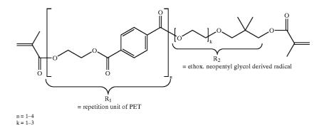
**[0035]** Preferred binders are those that are obtainable from glycolyzed aromatic polyester such as polyethylene terephthalate (PET). These binders are suitable as reactive components for reactive acrylic systems, more specifically for adhesive, coating and flooring compositions with:
