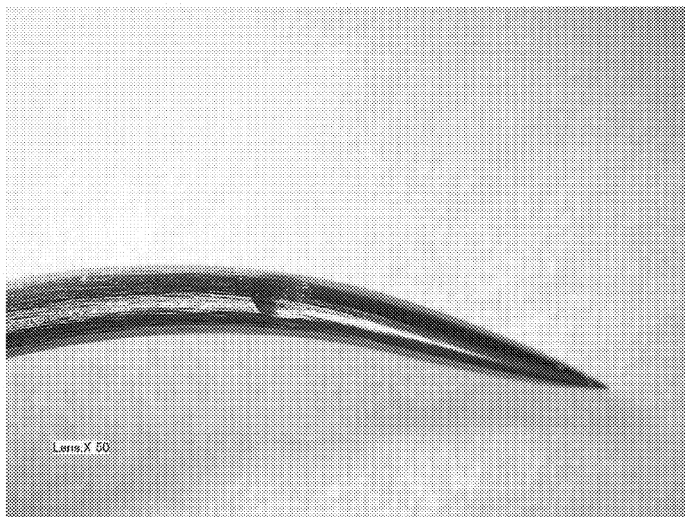
CT-1 Needle Cured at 100°C for 1 Hour.
