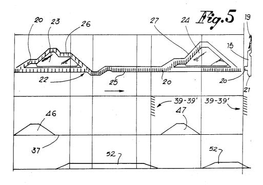
DEVICE SELECTING THE NEEDLES ON THE DIAL PLATE OF EITHER SINGLE OR MULTIPLE FEED, SINGLE CYLINDER CIRCULAR KNITTING MACHINES FOR THE MANUFACTURE OF RIBBED FABRIC
