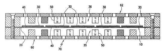
(57) **Abstract:** Planar magnetic transducers and acoustic speakers incorporating the transducers wherein improved frequency performance with lower distortion of acoustic diaphragms of the transducers is obtained by forming the diaphragms of film materials (20) which are significantly more compliant than materials used to form electrical circuit patterns (30) on the diaphragm film materials (20)
