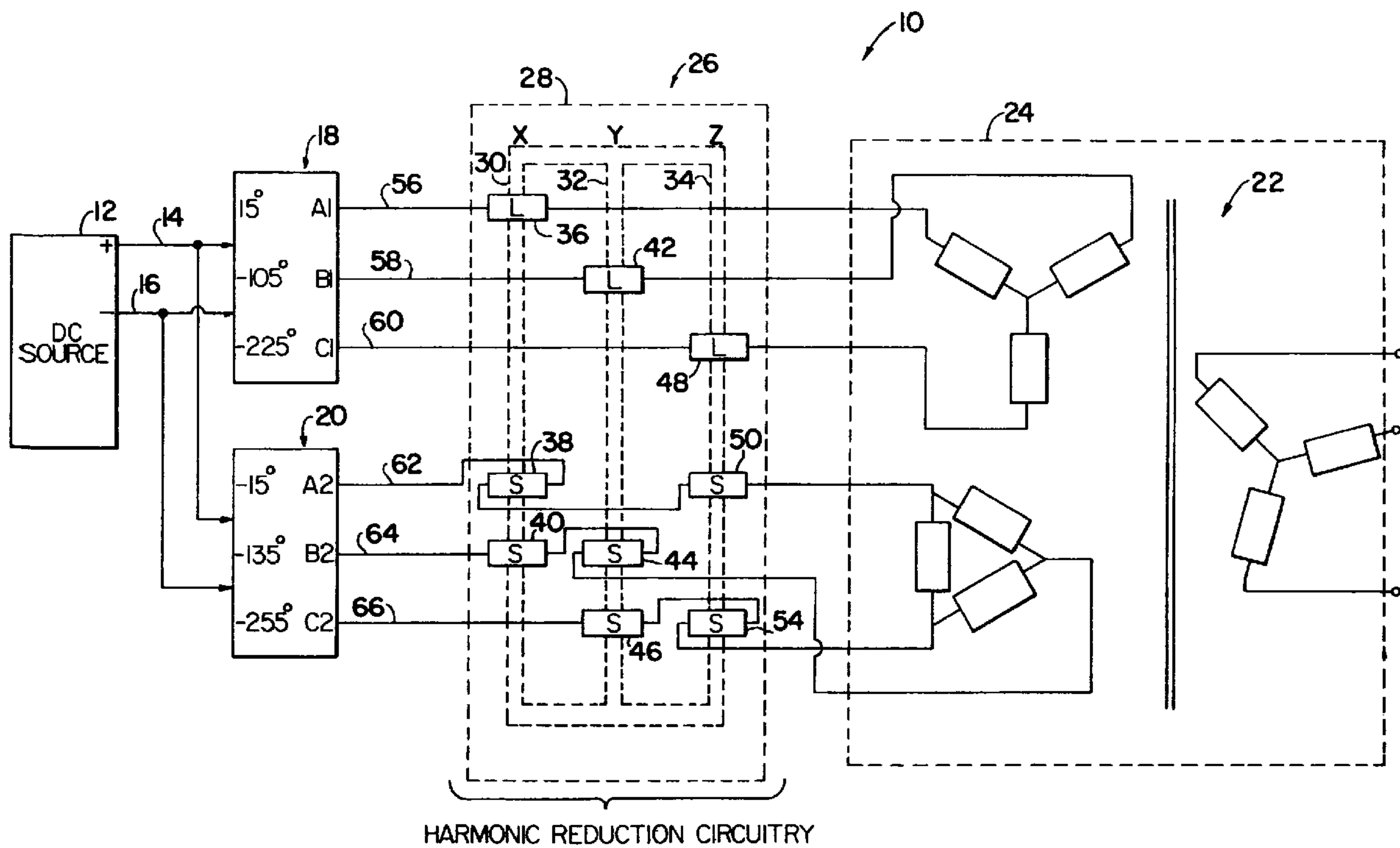
(57) A method for reducing the signal harmonics of the output fundamental signals of a three-phase inverter systems made up of an  $N$  number of inverter bridges achieves harmonic signal reduction by combining the outputs of immediately adjacent bridges separated by  $60^\circ/N$  relative to one another and then summing the combined sum signal with the outputs of the next immediately adjacent bridge.
