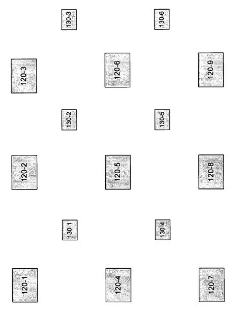
Larger contact pads 120 are connected to package. Smaller contact pads 130 are unconnected (as there are no stacked die).
