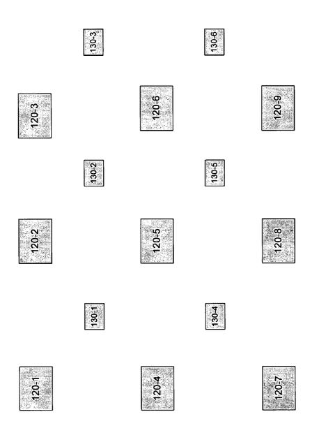
Larger contact pads 120 are connected to package. Smaller contact pads 130 are connected to stacked cache die.
