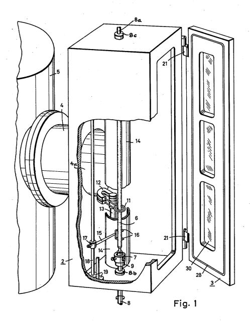
DEVICE FOR CRUCIBLE-FREE ZONE MELTING
