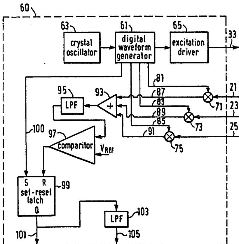
APPARATUS AND METHOD FOR PROCESSING SIGNALSOBTAINED FROM A POSITION ENCODER
