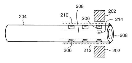
(57) Abstract: Method producing a coated medical support device capable of insertion into the body, the method including the procedures applying a coating to a section of a work piece (210), position the work-piece (210) in the vicinity of an electromagnetic field generator, and substantially proximate a forming mandrel (204), inducing electromagnetic forces in the work-piece (210) which accelerate the work-piece (210) toward the forming mandrel (204), and
