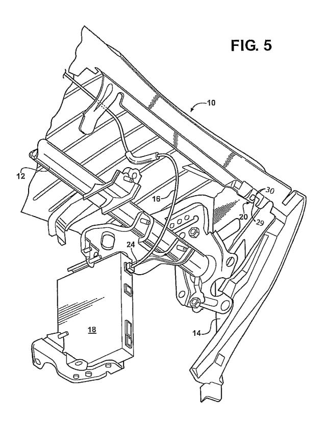
Method of Aiding the Attachment of a Cable to an Electrical Component Wherein the Cable is Attached to a Substrate and the Electrical Component is Mounted onto a Vehicle Body Structure.
