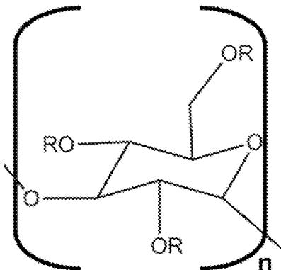
5 Regarding the formula of this structure, n can be at least 6, and each R can independently be an H or an organic group. Furthermore, the poly alpha-1,3-glucan ether compound has a degree of substitution of about 0.05 to about 3.0. Significantly, a poly alpha-1,3-glucan ether compound herein can be an alkyl ether and/or hydroxyalkyl ether derivative of poly alpha-1,3-glucan.
