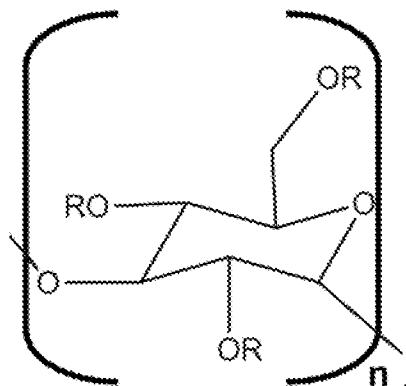
20 Regarding the formula of this structure, n can be at least 6, and each R can independently be a hydrogen atom (H) or an organic group. A poly alpha-1,3-glucan ether compound herein has a degree of substitution of about 0.05 to about 3.0.
