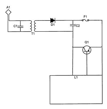
(57) Abstract: In regular operation, the tag receives energy from antenne (A1), which is fed resonant circuit comprising of capacitor C1 and an inductor which is a portion of (T1). Energy captured from the secondary winding of (T1) is rectified by diode (D) and filtered by capacitor (C2). The energy collected is used to power the tag. It should be noted that this power supply arrangement is but one simplified arrangement of many known methods of providing power to the tag.
