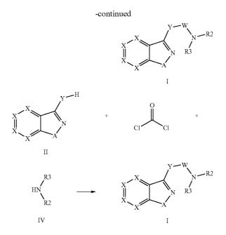
**21.** A process for preparing a compound of general formula I wherein R3 is hydrogen (formula Ia) as claimed in claim 1, which comprises reacting an azole of formula II with an isocyanate of formula V, O=C=N-R2, as summarized in the following reaction scheme, in which the substituents are as defined in claim 1.
