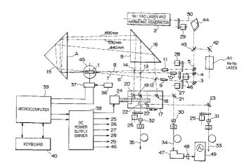
damage. To achieve this object, a multi-wavelength laser apparatus including an optical parametric oscillator having a nonlinear optical crystal and an excitation laser light source includes mirrors for dividing a laser beam emitted from the excitation laser light source into at least three optical axes, and a ring type resonator which simultaneously inputs the laser beams divided by these mirrors at different angles to
